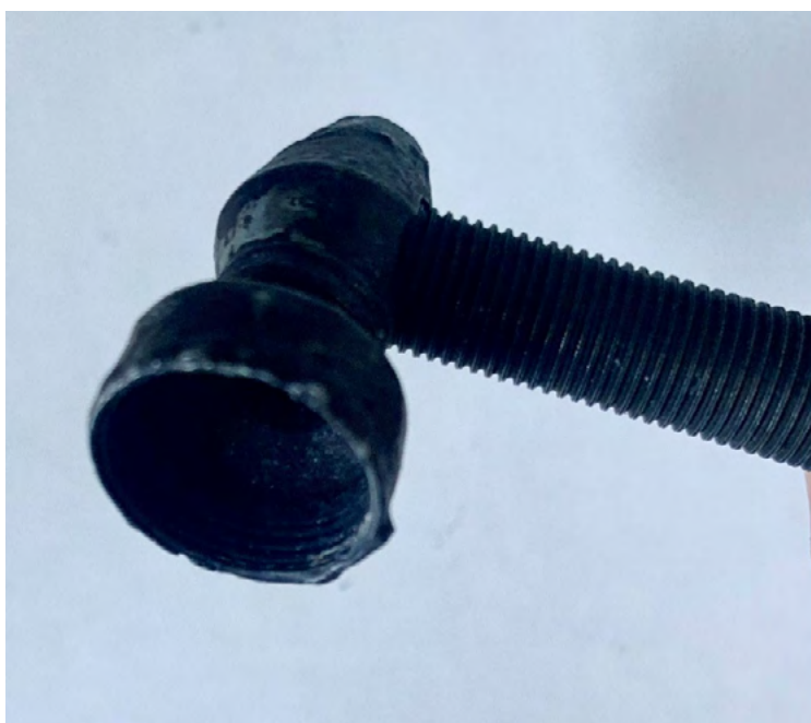
Figure 3 and 4: Crack pipe that had been used for less than two weeks.
